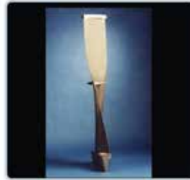
Compressor Blade Repaired by LENS System
