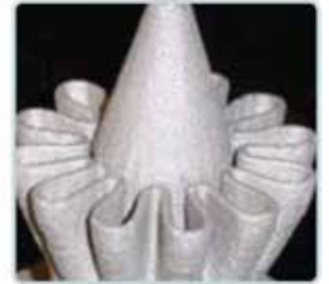
Exhaust Duct Fabricated by LENS System
